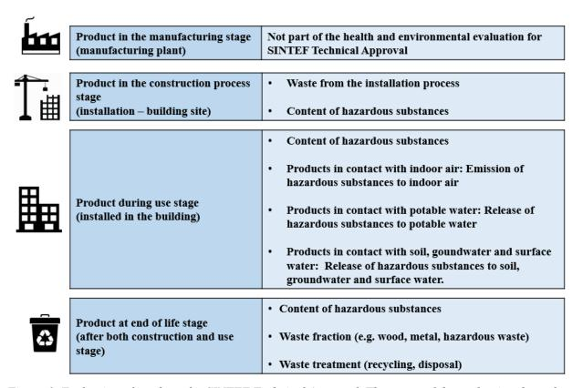
Figure 1. Evaluation of products for SINTEF Technical Approval. The extent of the evaluation depends on the placement in the building.
