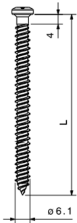
Fig. 19 CS-6,1 Concrete screw (with flat or sharp point)
