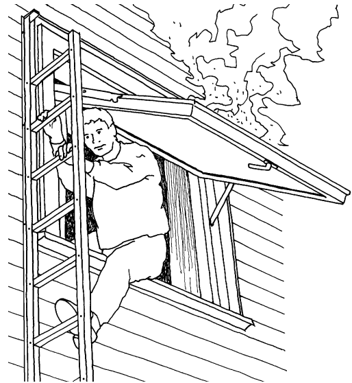
Fig. 1 Hardhaus veggstige utfelt for bruk under rømming.
