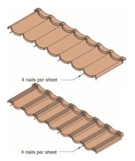
Fig. 4 Nailing of the sheets
